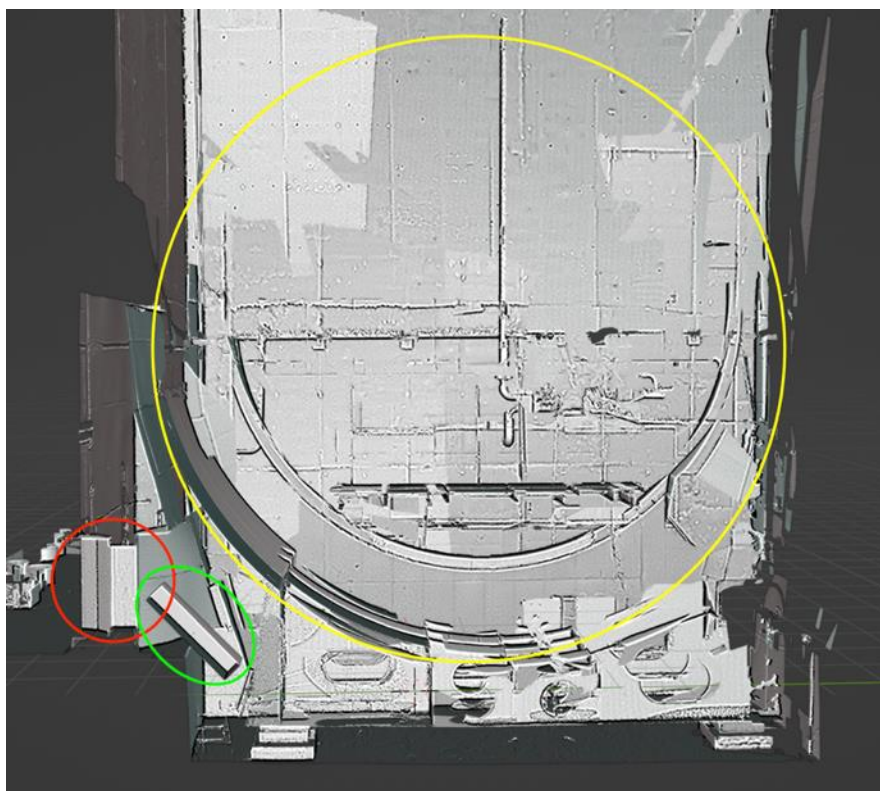
Figure 30. Scale of the entrance (marked with red), a hodoscope (marked with green) in comparison to the 346B reactor (marked with yellow). The reactor area seems hollow due to the 3D reconstruction method.
