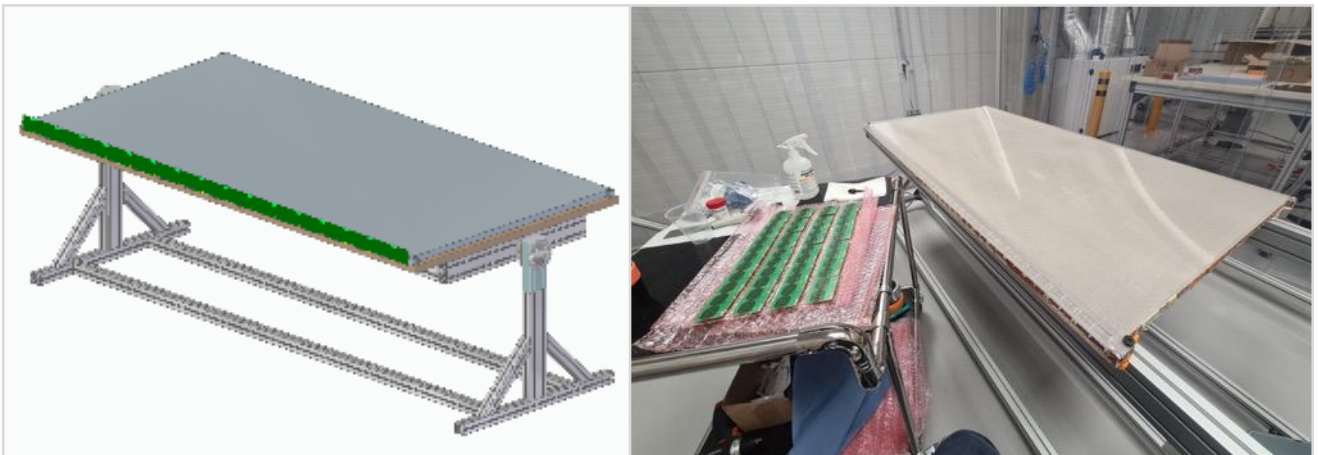
Figure 4. An assembly table inside the clean room for mounting SiPM arrays and mirrors. The table plane can be adjusted from horizontal to vertical direction.
