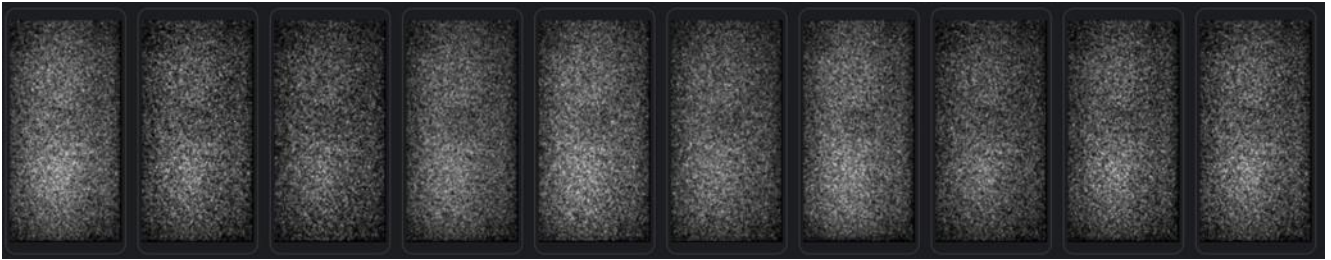
Figure 25. The reconstruction of test exposure of the second hodoscope (detector No. 2.) with different filtering ranges. Voxel size 1 cm. Two lead bricks were placed side by side and exposure time was 60 minutes.
