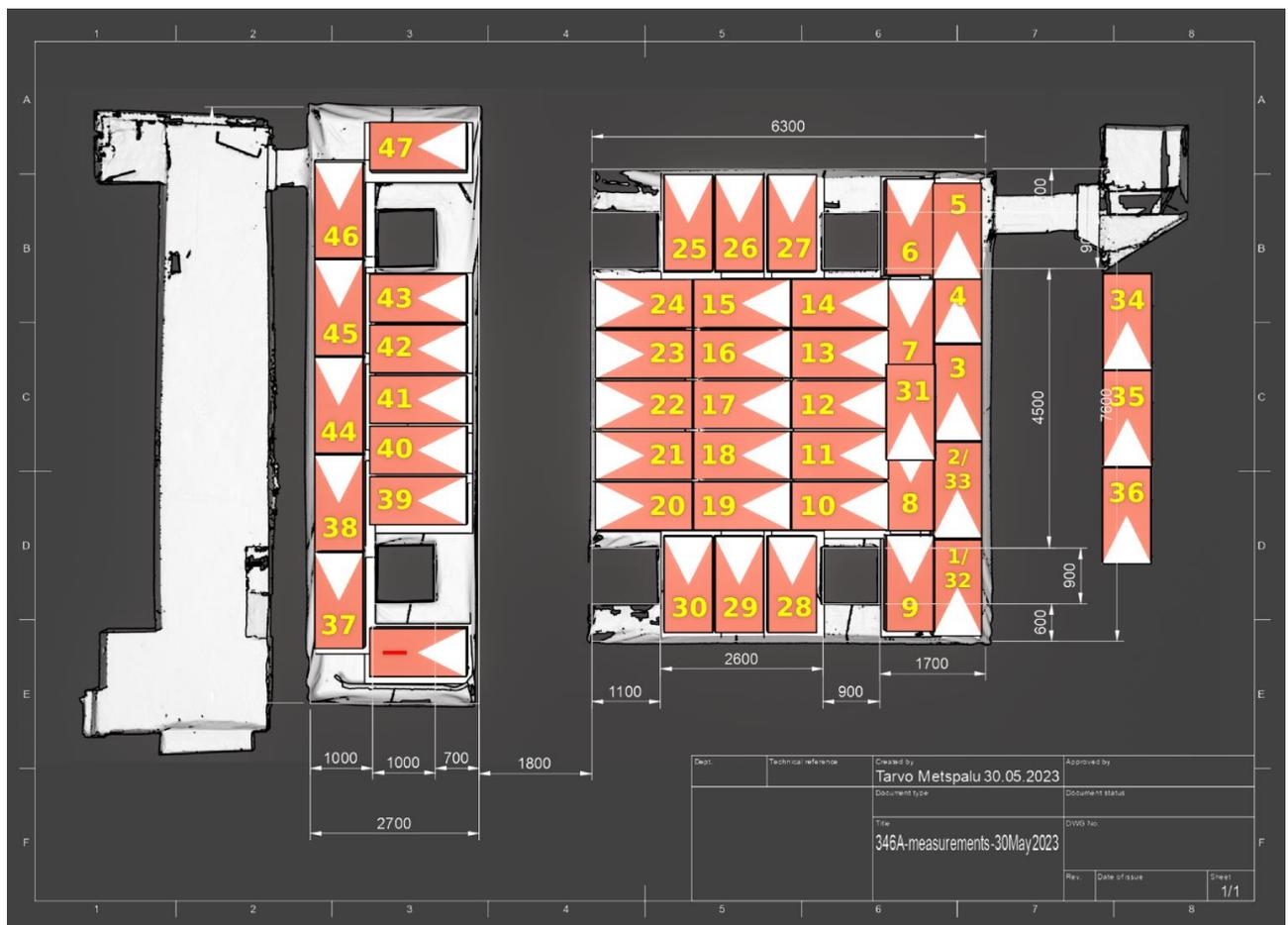
Figure 5-6. Measurement plan of the 346A reactor, where 47 different hodoscope measurement positions have been indicated. Some additional measurements were made at positions 1 and 2, respectively, as the initial flux was greater due to gamma rays, as previously expected.
