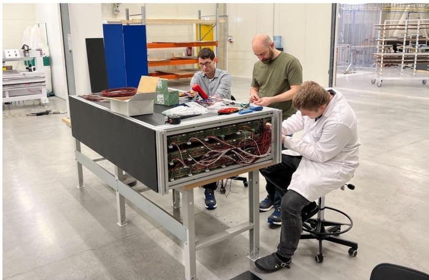
Figure 2-3. Full-scale hodoscope assembly: cabling and checking multiplexing connections
