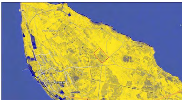
Figure 7.23. NDPI values around the PAL site. No impact of the temporary flooding (blue end of the colour palette) can be seen nearby the site. Sentinel 2 NDPI values for 2020.04.07 from the EstHUB Estonian Landboard.
