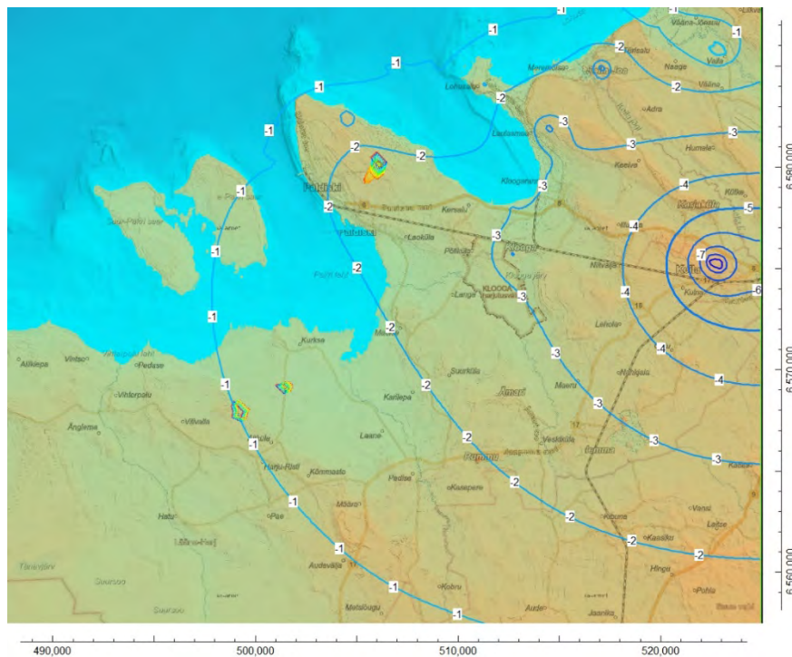
Figure 6.8. Simulated hydraulic head in Sämi aquifer (isolines) and contaminant transport from the potential repository sites (coloured pathlines).
