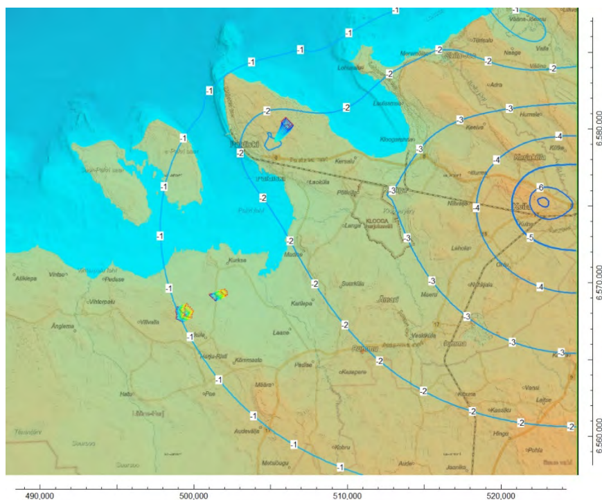
Figure 6.9. Simulated hydraulic head in Cambrian-Vendian aquifer (isolines) and contaminant transport from the potential repository sites (coloured pathlines).
