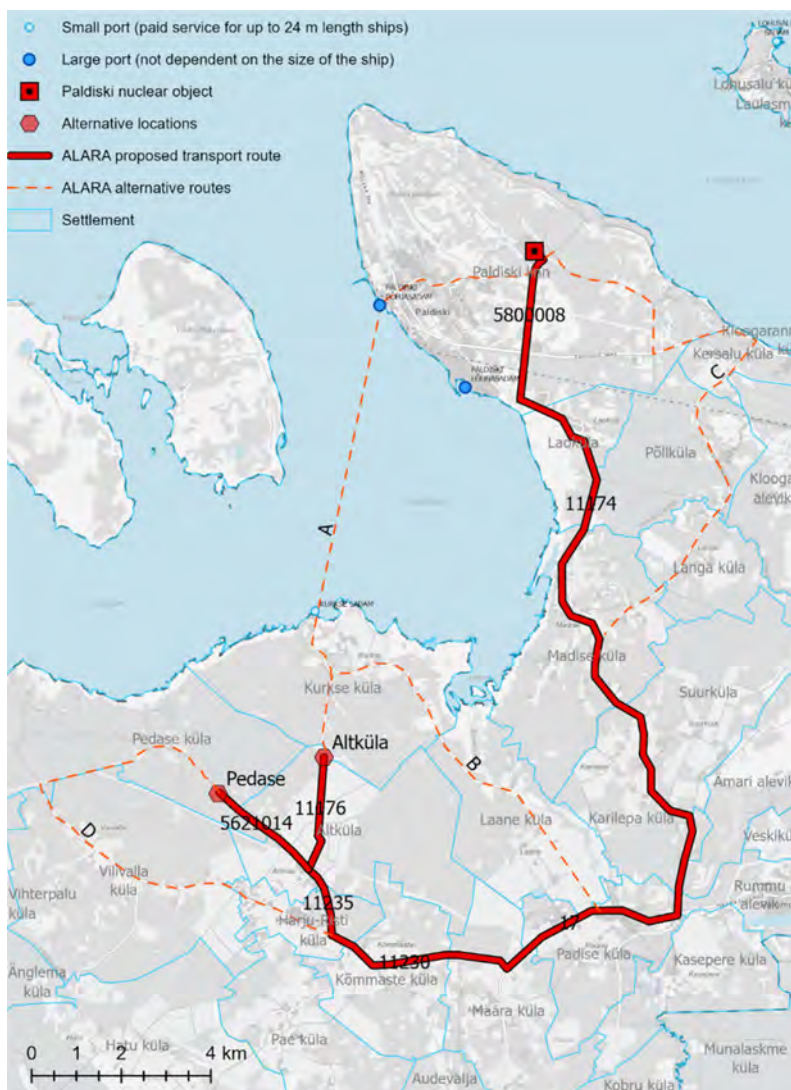
Figure 15.1. Optimal transport routes and alternative routes for radioactive waste transport from FPNS to Pedase and Altküla sites and traffic frequencies on the routes.
