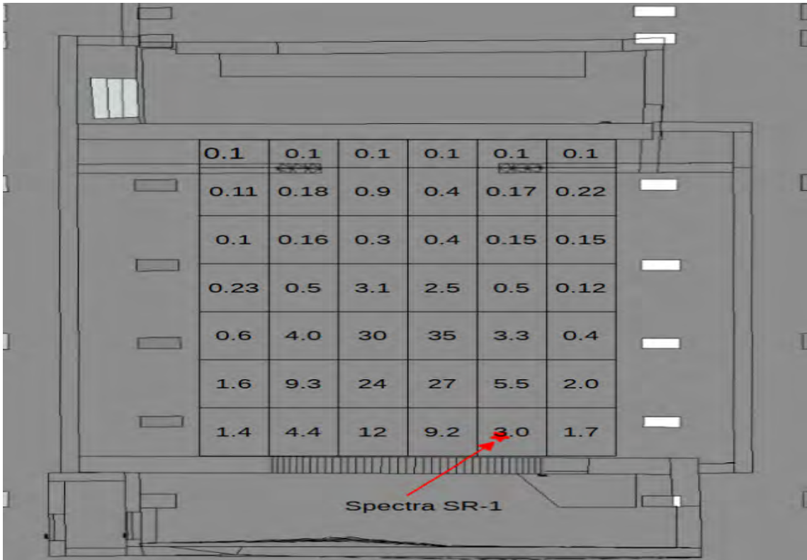
Fig. 3. Gamma-ray dose rates ( \mu\text{Sv/h} ) in the room under the reactor No. 1 1 m above the floor
