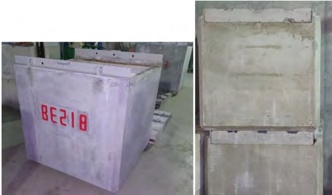
Figure 2.6. Standard concrete containers with cemented waste is predominant container type.
