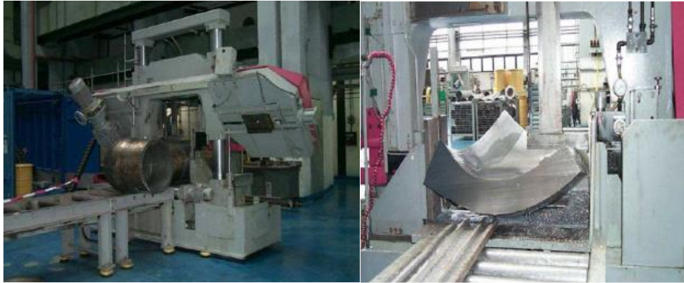
Examples of machine tools used for decommissioning (Behringer horizontal band saw)
