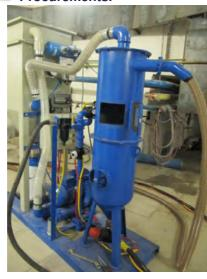
Vacuum blasting unit (for decontamination)
