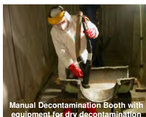
Technical cleaner used for discharging an ion exchange resin
