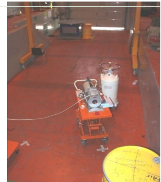
Gamma spectrometry measurements on radioactive drums at CSA
