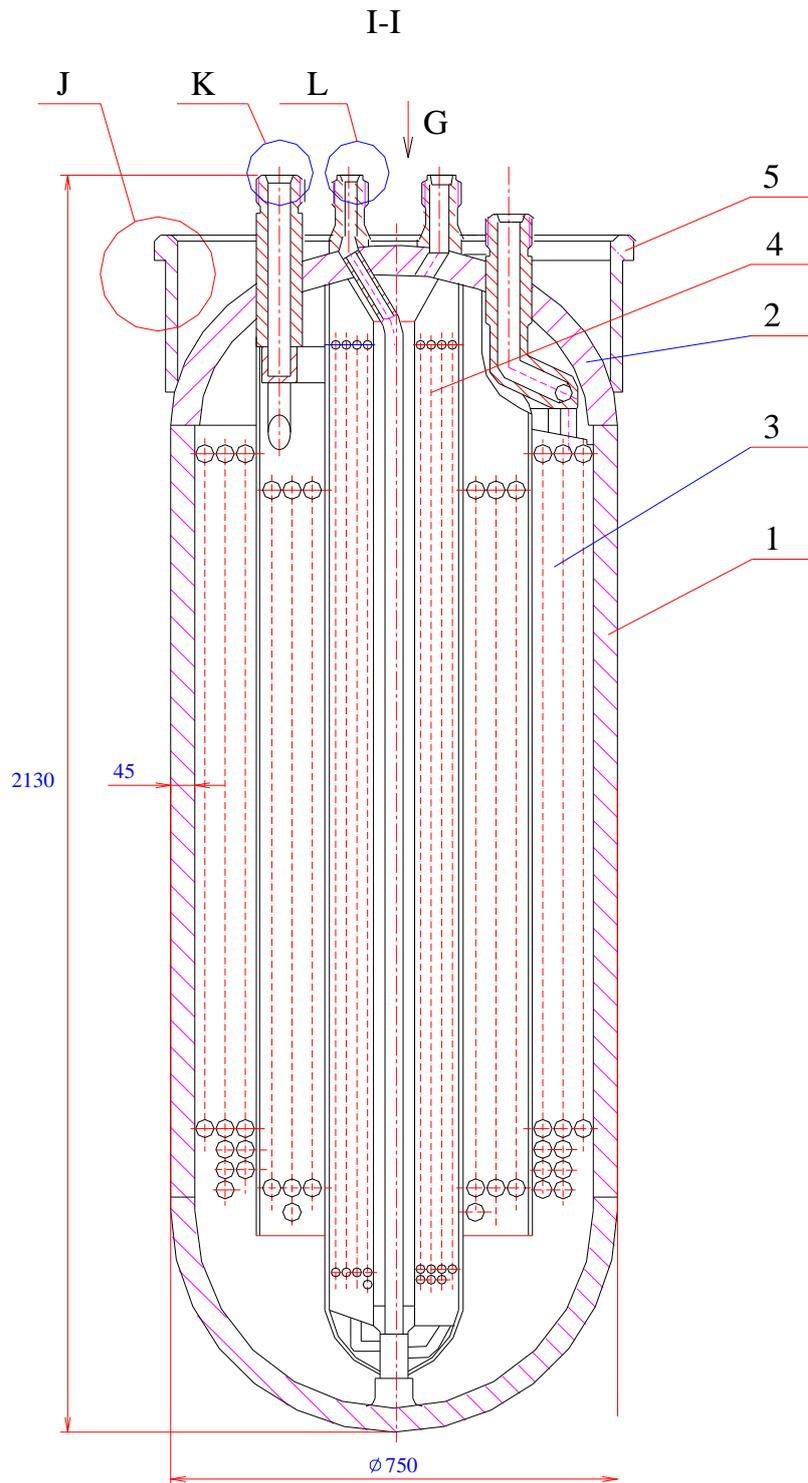
1 - casing; 2 - cover; 3 - cooler; 4 - recuperator; 5 - support.
