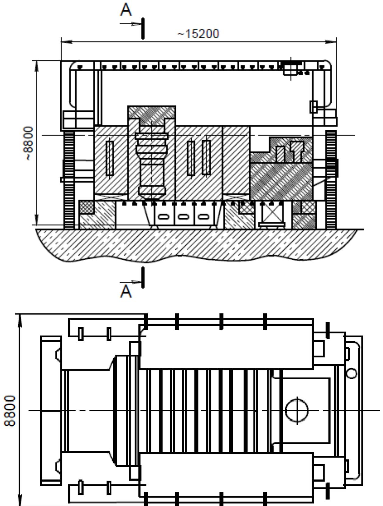
Figure 19 (a, b, c). Reactor Stand 346B
