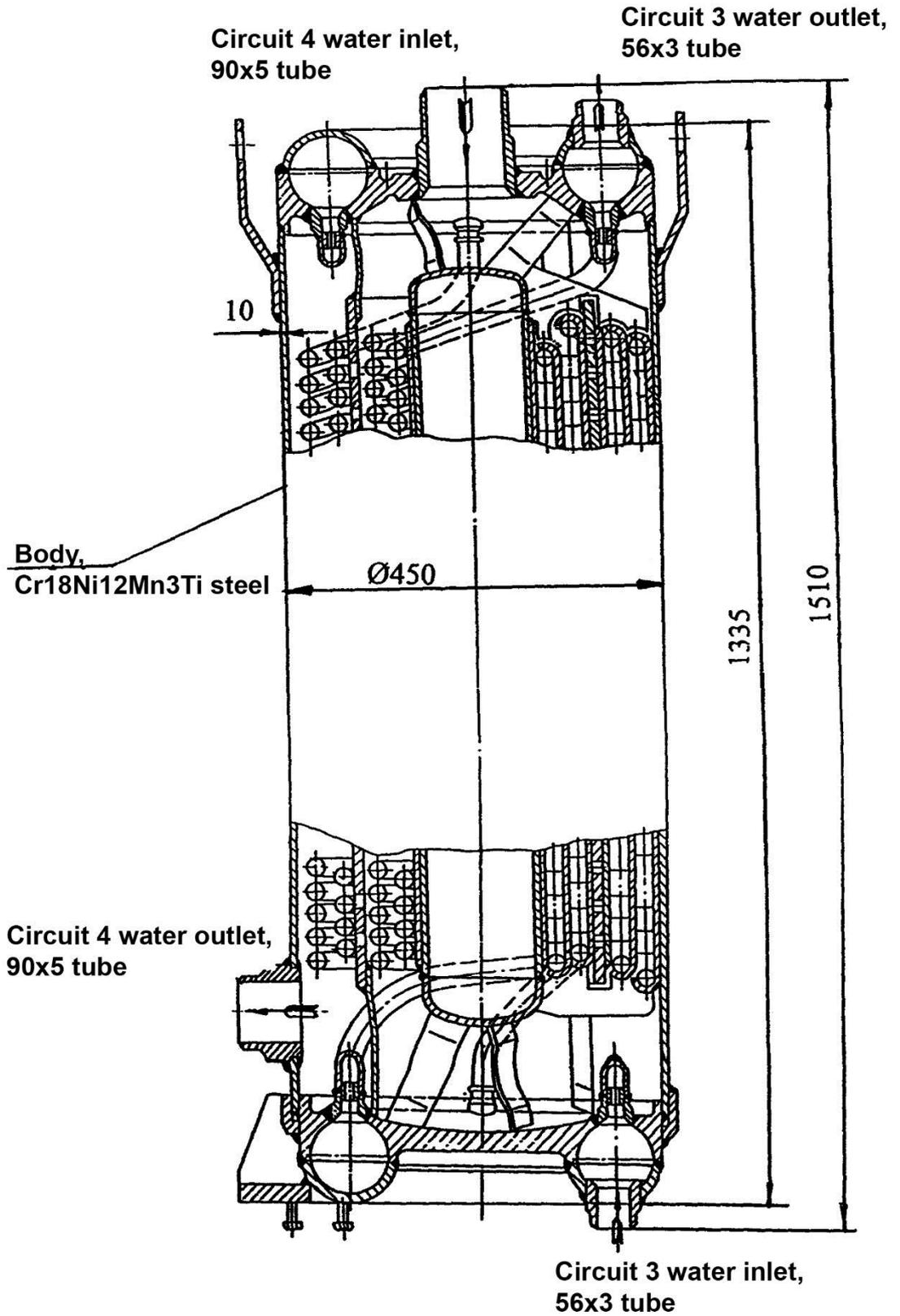
Figure 10. Circuits 3-4 VP 2-1-0 heat exchanger
