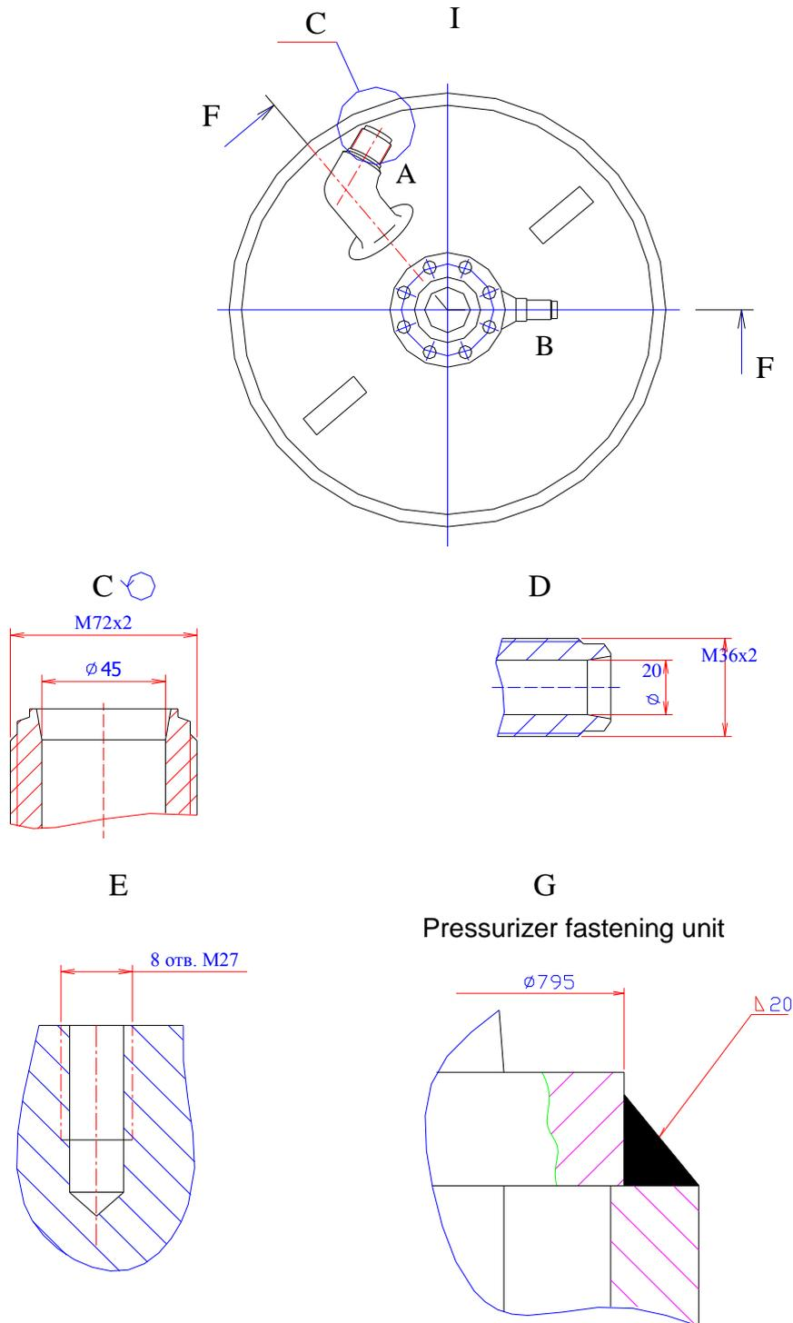
A - water inlet-outlet; B - gas inlet-outlet.
