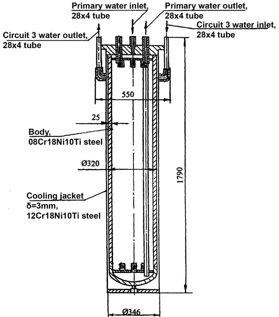
Figure 6. Radioactivity filter
