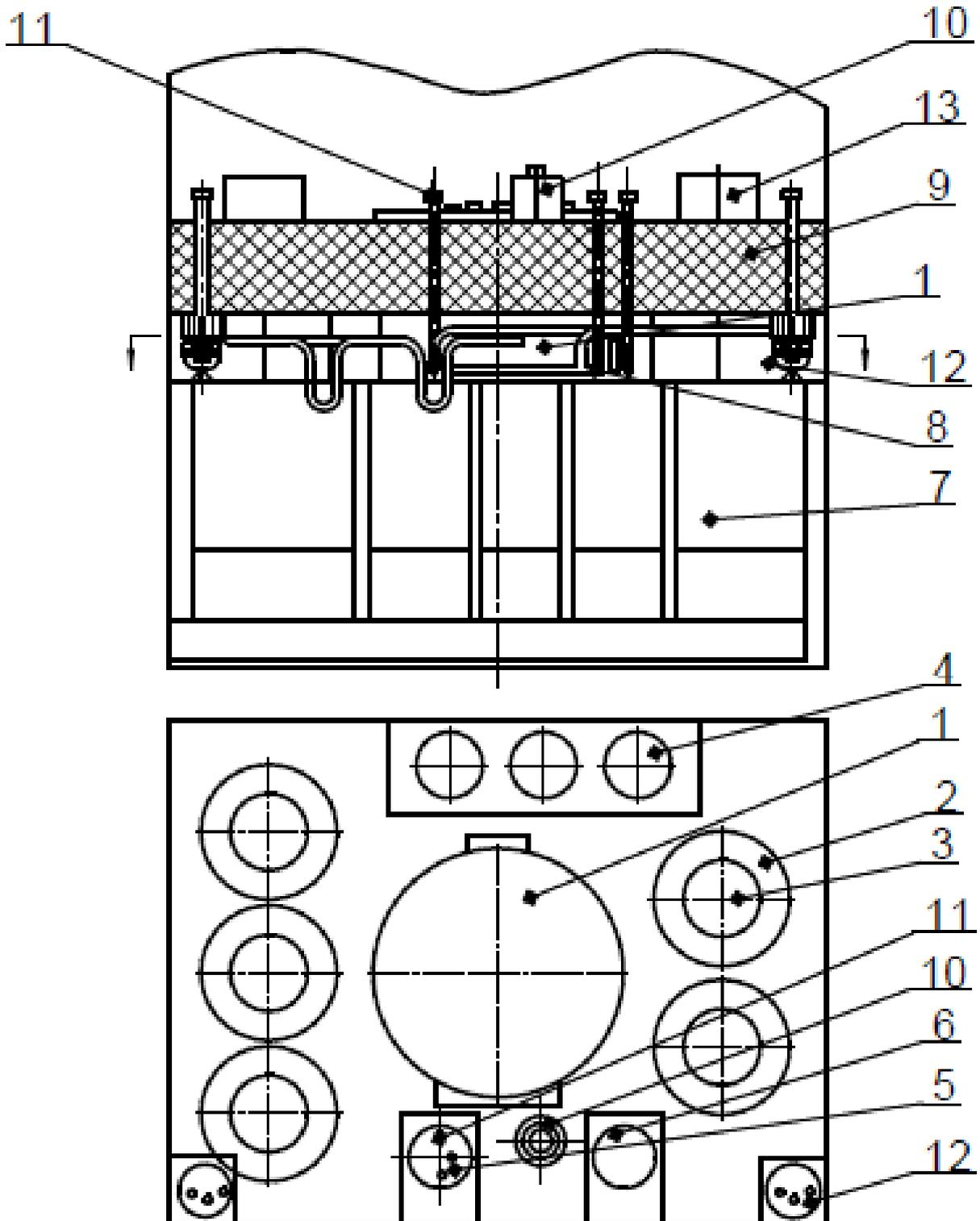
1 reactor; 2 steam generator; 3 primary circuit pump; 4 primary circuit pressurizer filter refrigerator; 5 valve unit; 6 primary fluid filter; 7 shield tank; 8 primary pipings; 9 bioshield; 10 cool-down pump;
