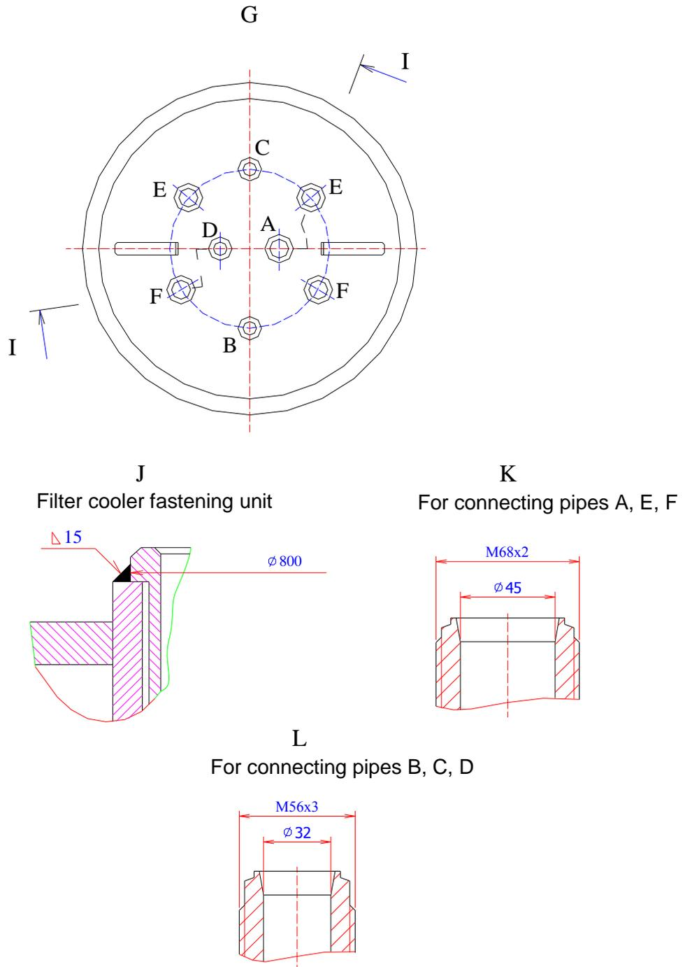
A - recuperator inlet; B - cooler outlet; C - recuperator inlet after filter;
