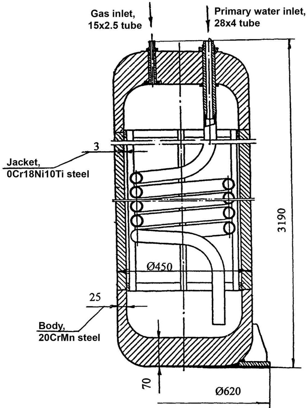
Figure 4. Pressurizer (cylinder), assembly 13
