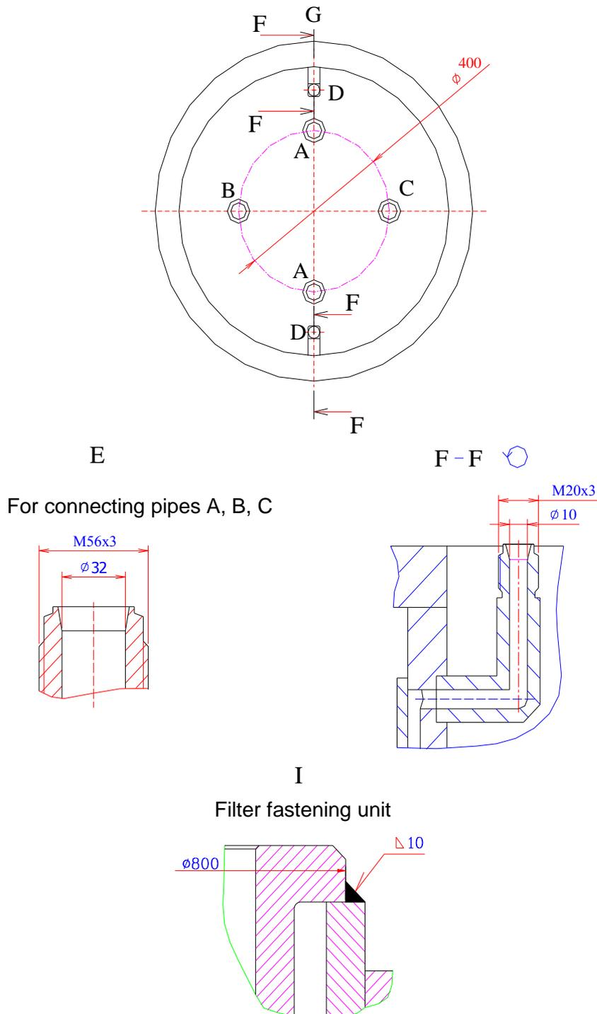
A - water inlet; B - water outlet; C - loading-unloading; D - III circuit inlet-outlet.
