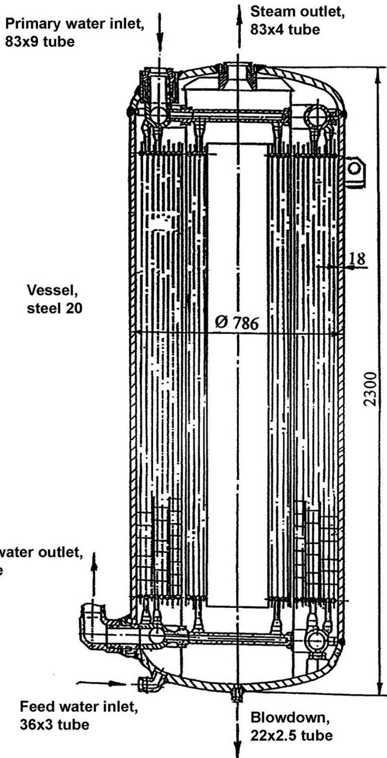
Figure 1. PG-14T steam generator chamber
